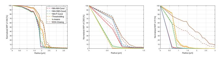
Figure 7: Simulated mercury intrusion porosimetry of active material (left), CBD (center) and pore space (right) for the two-layer cathode (dashed curves) and the single-layer cathode (solid curves).
