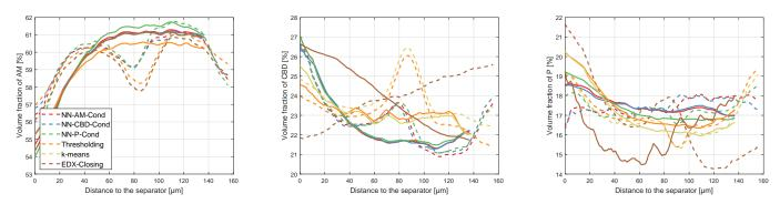
Figure 10: Volume fraction of active material (left), CBD (center) and pores (right) in dependence of the distance to the separator for the two-layer cathode (dashed curves) and the single-layer cathode (solid curves).
