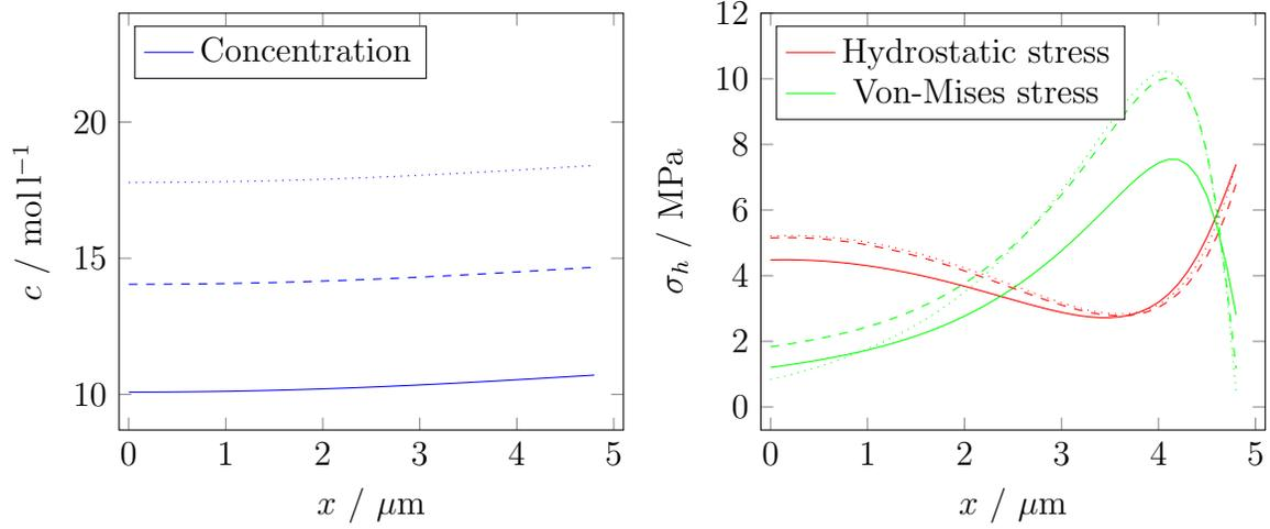
**Figure 3:** Radial-symmetric solution of (i) lithium-ion concentration and (ii) hydrostatic stress and von-Mises stress in a spherical particle for states of charge 40%, 55% (dashed) and 70% (dotted).
