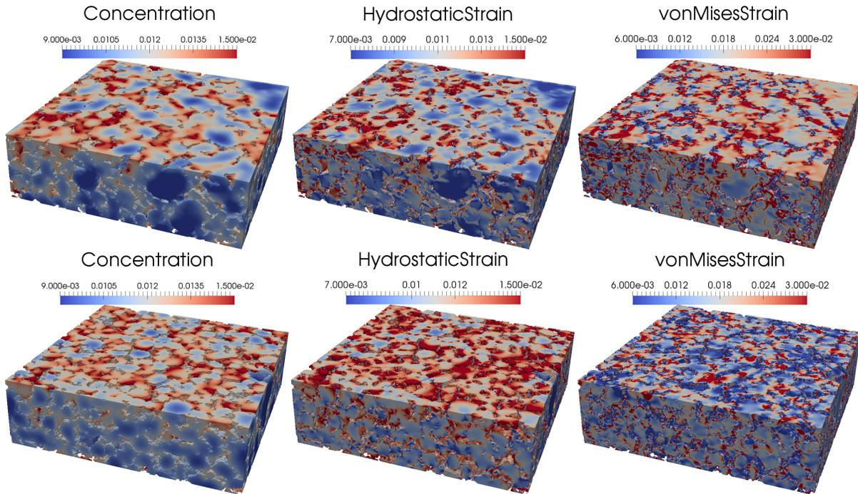
**Figure 4:** Full-field solution of lithium-ion concentration, hydrostatic stress and von-Mises stress in both tomographic (top) and simulated (bottom) microstructures.
