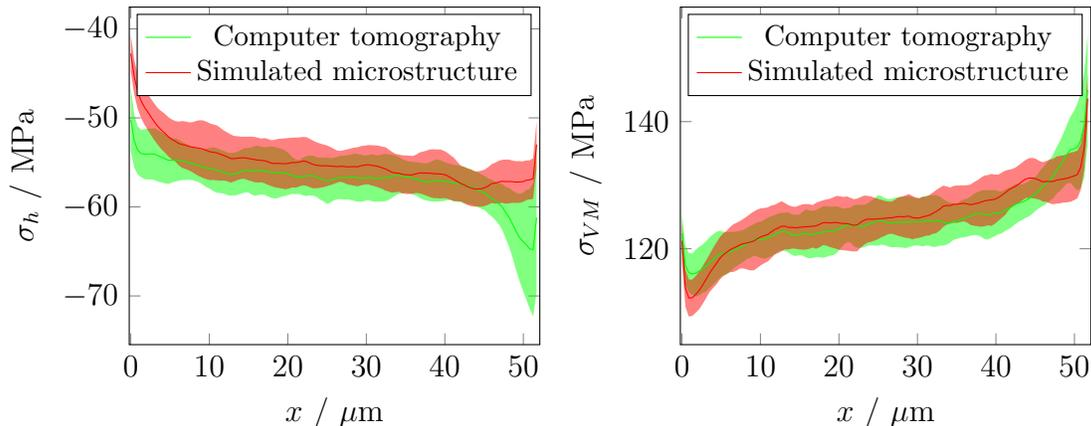
**Figure 5:** Comparison of the hydrostatic stress (left) and the von-Mises stress (right) for SOC=40% in the thickness direction. Plotted is the mean as well as  $\pm 1$  standard deviation.
