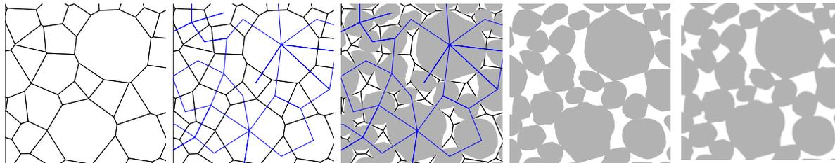
**Figure 1:** 2D sketch showing the individual steps of the stochastic microstructure model proposed in [2]. (i) Decomposition of the sampling window into convex polytopes. (ii) Construction of a connectivity graph. (iii) Modeling of particles according to the constraints given by the connectivity graph. (iv) The auxiliary tools are deleted. (v) A morphological closing is performed to mimic the effect of binder. Reprinted from [2], with permission from Elsevier.
