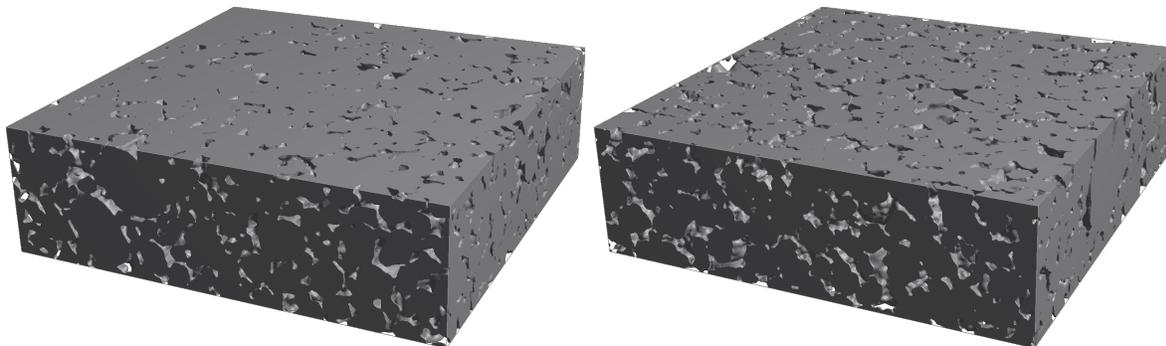
**Figure 2:** Left: CT image. Right: Simulated structure using the calibrated stochastic model.
