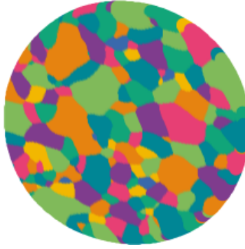
Figure 3: 2D slice through the 3D dataset of 99.9% pure iron [109], provided by H. F. Poulsen. The image size is 280 \times 320 \times 256 with a voxel edge length of 1.54 \mu\text{m} .
