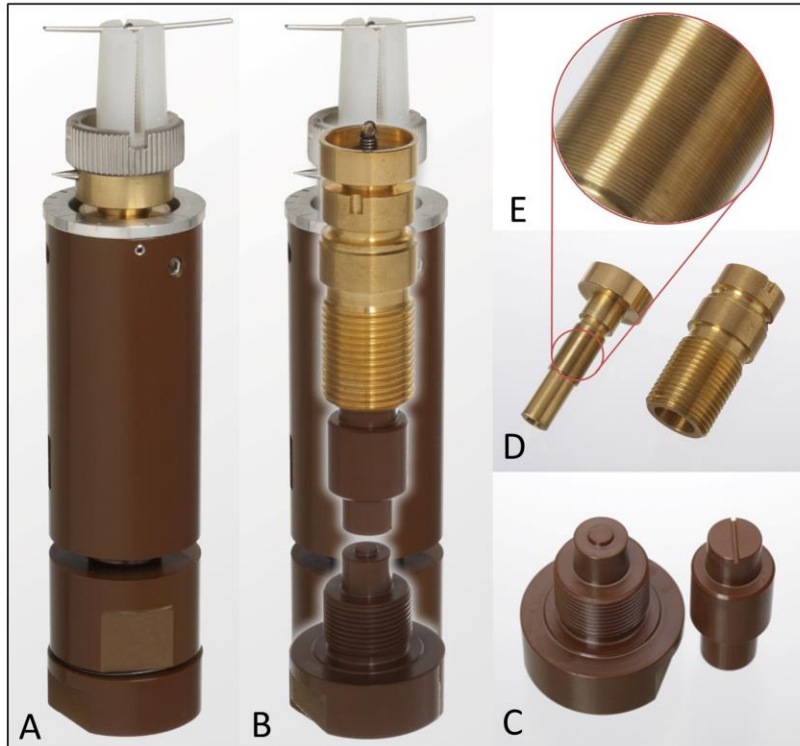
Figure 2. Compression device used for high resolution tomography of circular GDL samples. A: total view. B: transparent total view revealing interior details of the construction. C: Sample holder basis (left) and compression punch with integrated channel structure mimicking the flow field channel geometry (right). D: Hollow adjustment screw and sleeve made of brass. E: Detail of the adjustment screw showing the male ultra-fine thread (pitch = 200 \mu\text{m} ).
