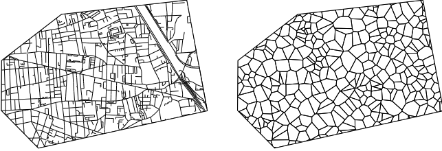
Fig. 4. A real road system (528 crossings, 324 quarters, 849 street segments and 97 km total street length) is replaced by a simple random PVT giving in the average (585 crossings, 293 quarters, 878 street segments and 82 km total street length)
