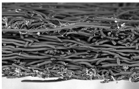
Fig. 5 Profile of a nonwoven-type GDL
