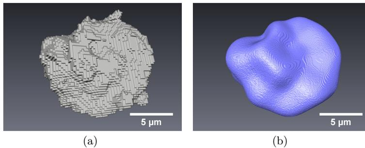
**Fig. 3.** Example of a particle from an energy cell anode. Segmented particle from tomographic image (a) and approximation of the particle with a truncated series of spherical harmonics for  $L = 10$  (b). Reprinted from [7] with permission from Elsevier.
