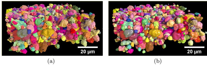
**Fig. 2.** Comparison of the result of structural segmentation and approximation of particles by spherical harmonics. Particle system before (a), and after approximation by spherical harmonics (b). Reprinted from [7] with permission from Elsevier.
