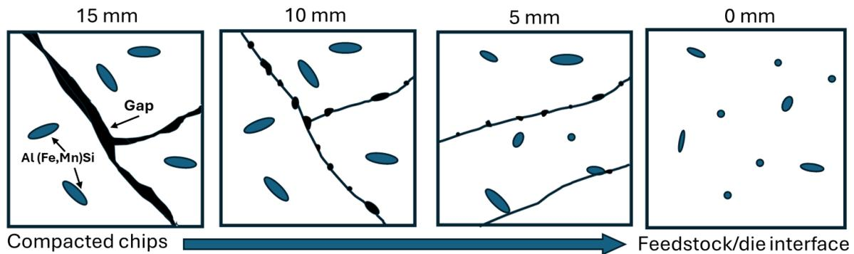
Figure 8. Progressive compression and bonding of irregular chips during the FE/FC process, evolving from weak initial interfacial contacts to full consolidation near the die interface.
