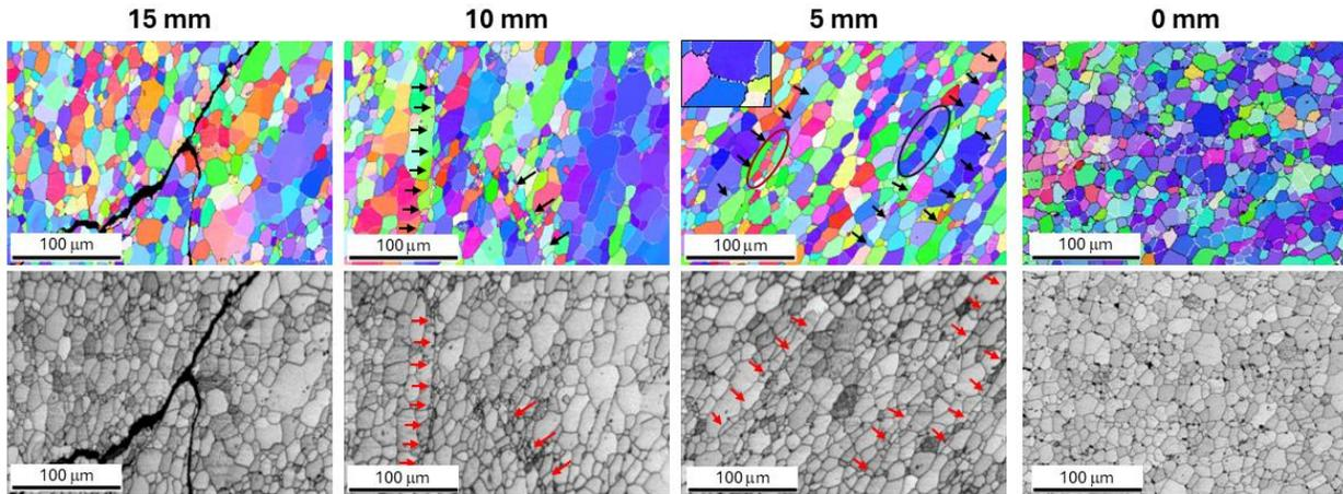
Figure 4. EBSD maps and SEM grain boundary contrast images were obtained at 15, 10, 5, and 0 mm positions. The arrows in the maps show chips boundaries, while highlighted ellipse show elongated grains because of high strain resulting from friction and compression.
