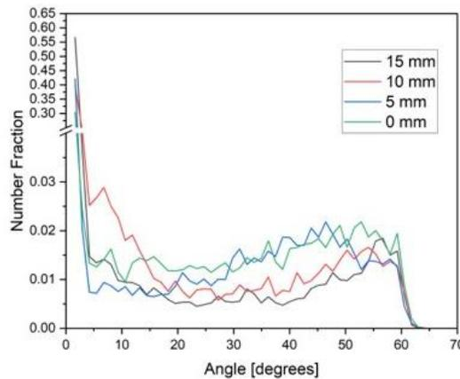
Figure 7. Grain boundaries misorientation angles distribution at distances of 15, 10, 5, and 0 mm, showing the relative fractions of LAGBs and HAGBs
