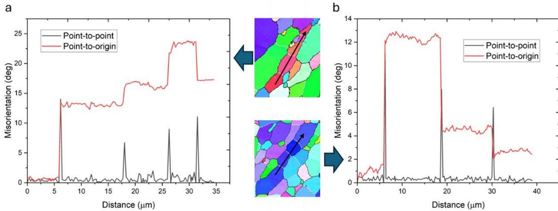
Figure 6. Misorientation along the arrows in the EBSD maps, indicated by (a) red ellipse and (b) black ellipse in region 5 mm in Fig. 4.
