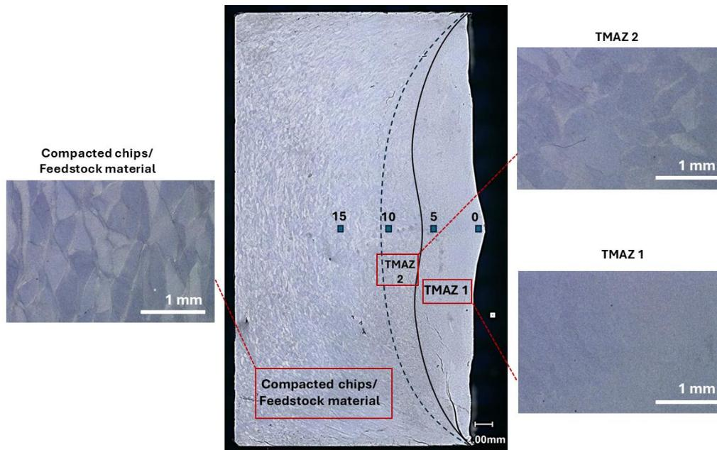
Figure 2. Macrograph of the residual material after friction extrusion of Al chips at distances of 15, 10, 5, and 0 mm from the die–material interface, where 15 mm corresponds to the compacted chip region and 0 mm is adjacent to the die interface.
