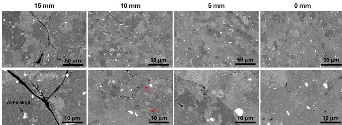
Figure 3. Micrographs taken from the base material interface towards die-feedstock interface at 15 mm, 10 mm, 5 mm, and 0 mm, see Fig. 2.
