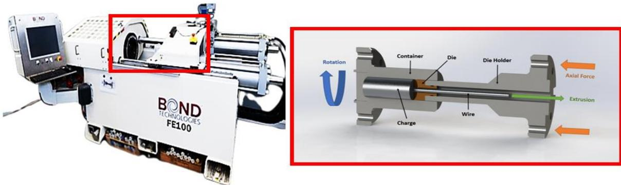
Figure 1. Illustration of Friction Extrusion Machine FE100 (Bond Technologies) and process principles [15].
