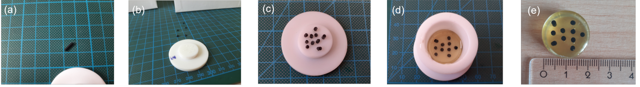
Figure 2: Correlative preparation procedure of CT and SEM-EDS samples: (a) hardened mixture of epoxy, sample and graphite, called an epoxy cylinder sample used for CT; (b) each epoxy cylinder sample is sliced into five disk pieces; (c) a total of ten pieces are obtained from two epoxy cylinder samples with two different size fractions, 63\ \mu\text{m} to 100\ \mu\text{m} and 100\ \mu\text{m} to 250\ \mu\text{m} ; (d) embedding the cut pieces into epoxy resin; (e) the resulting embedded sample which will later be re-embedded in epoxy, ground and polished to have the epoxy grain mount for SEM-EDS. The size of underlying square (b-d) is 10 mm.
