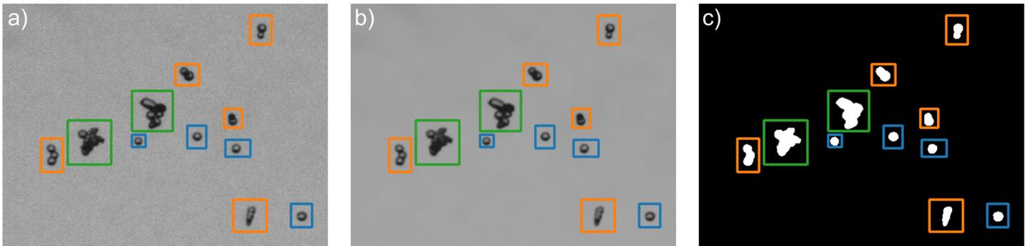
Figure 2: **Preprocessing of images.** a) Exemplary cutout of an image depicting particles/agglomerates of Experiment A at time step 50 min. b) Denoised (non-local means) of a). c) Corresponding phasewise segmentation of b). Exemplary, primary particles are highlighted in blue, chain-like agglomerates in orange and raspberry-like agglomerates in green.
