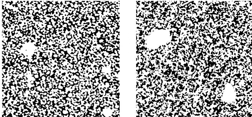
Figure 7: 2D cross-sections of tomographic data of sand (left) and simulated data (right).
