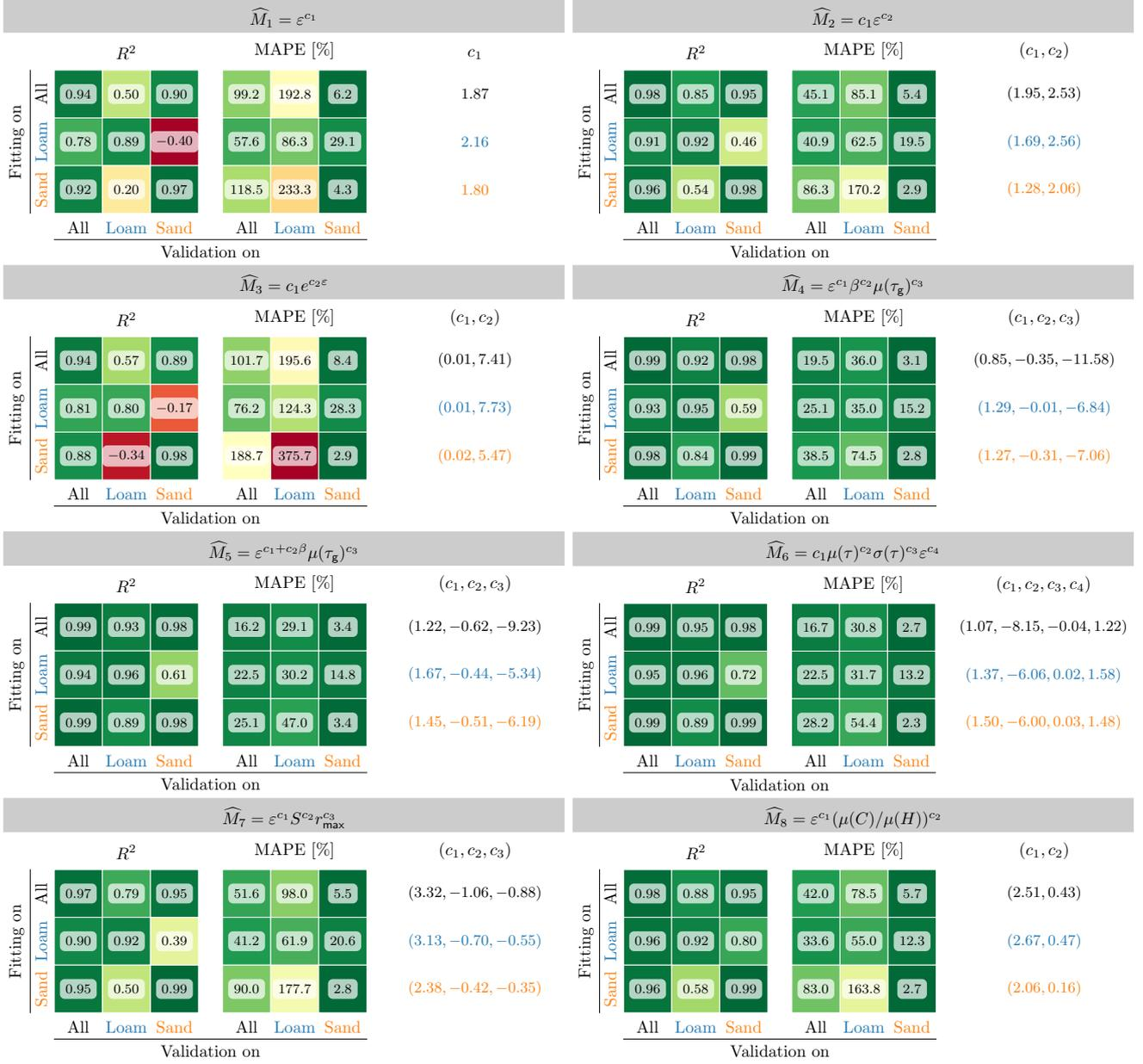
Figure 11: Validation scores  $R^2$  and MAPE obtained for the regression formulas considered in the present paper including the values for the corresponding regression parameters, where different data sets have been used for training/fitting and validation.
