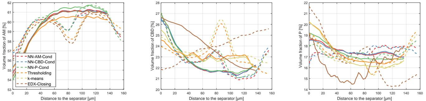
Figure 10: Volume fraction of active material (left), CBD (center) and pores (right) in dependence of the distance to the separator for the two-layer cathode (dashed curves) and the single-layer cathode (solid curves).
