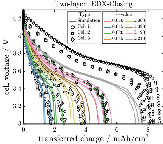
(a) Impact of the effective parameter  $\gamma$  on the simulated cell voltage for the EDX-Closing trinarization at  $6 \text{ mA/cm}^2$ . The target experiments are highlighted with filled green symbols.
