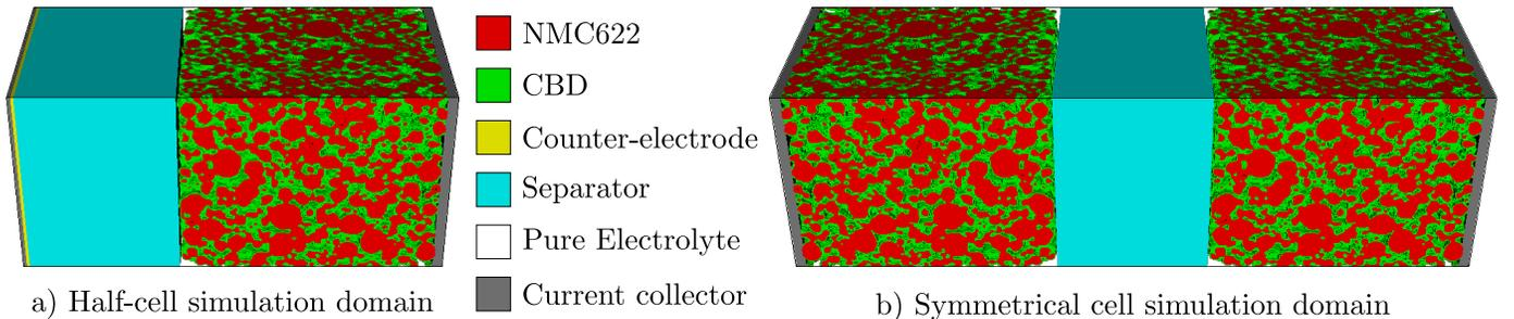
Figure 5: Simulation domains used for the two different types of electrochemical simulations.
