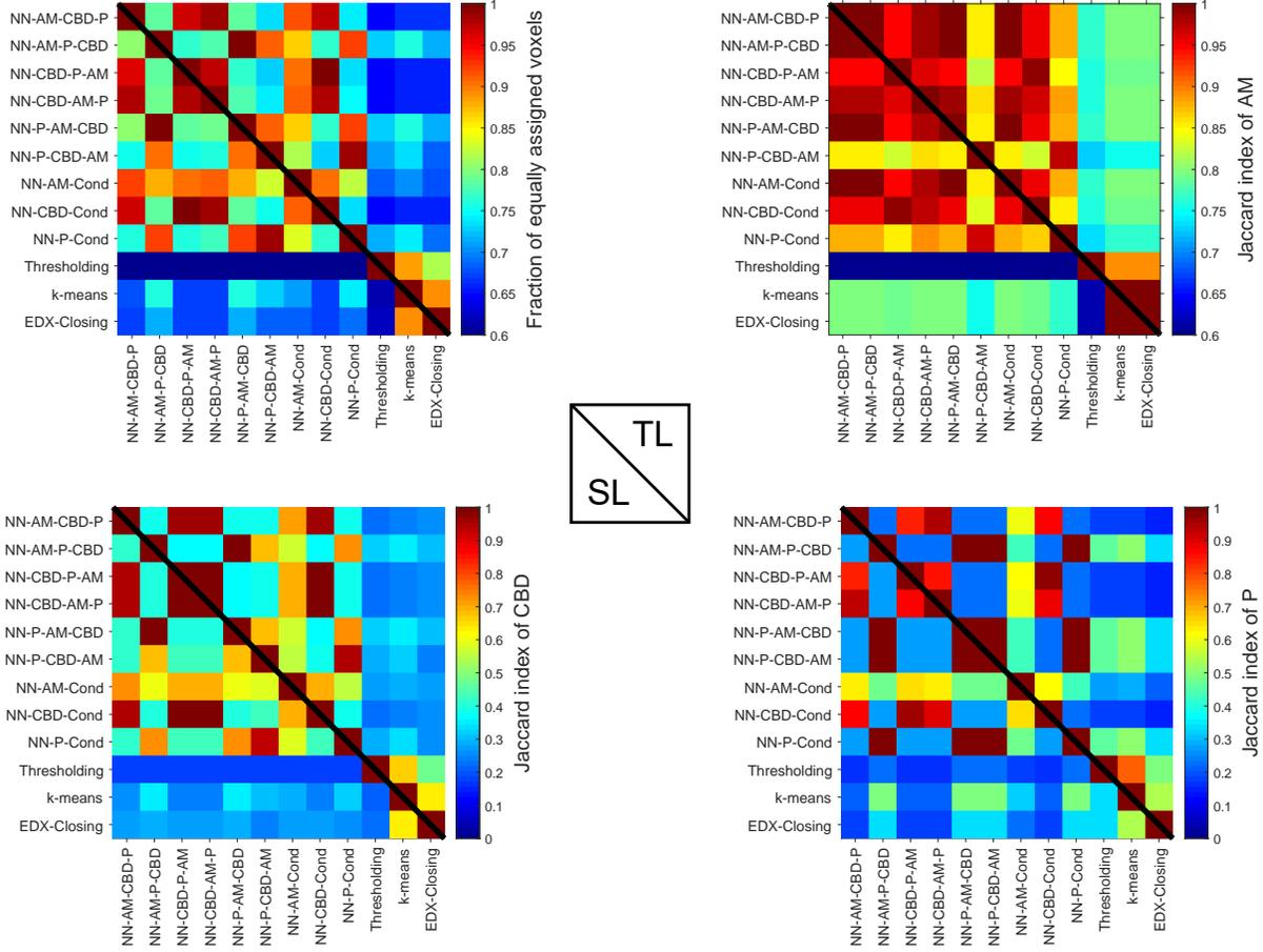
Figure 4: Fraction of equally assigned voxels (top left) as well as Jaccard index for active material (top right), CBD (bottom left) and pores (bottom right). Note that the entries above the main diagonal correspond to the two-layer cathode, whereas the entries below the main diagonal refer to the single-layer cathode. Due to the high accordance with regard to the spatial distribution of active material, the corresponding color bar only ranges from 0.6 to 1.
