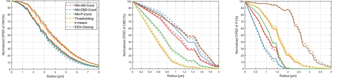
Figure 6: Continuous phase size distribution of active material (left), CBD (center), and pore space (right) for the two-layer cathode (dashed curves) and the single-layer cathode (solid curves).
