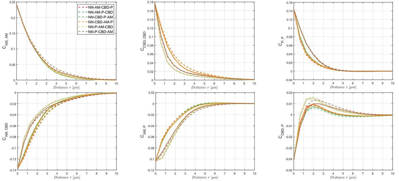
Figure S2: Top row: Centered two-point coverage probability function of active material, CBD and pore space (from left to right). Bottom row: Centered two-point coverage probability functions  $C_{AM,CBD}$ ,  $C_{AM,P}$  and  $C_{CBD,P}$  (from left to right). Note that dashed curves are used for the two-layer cathode, whereas the solid curves correspond to the single-layer cathode.
