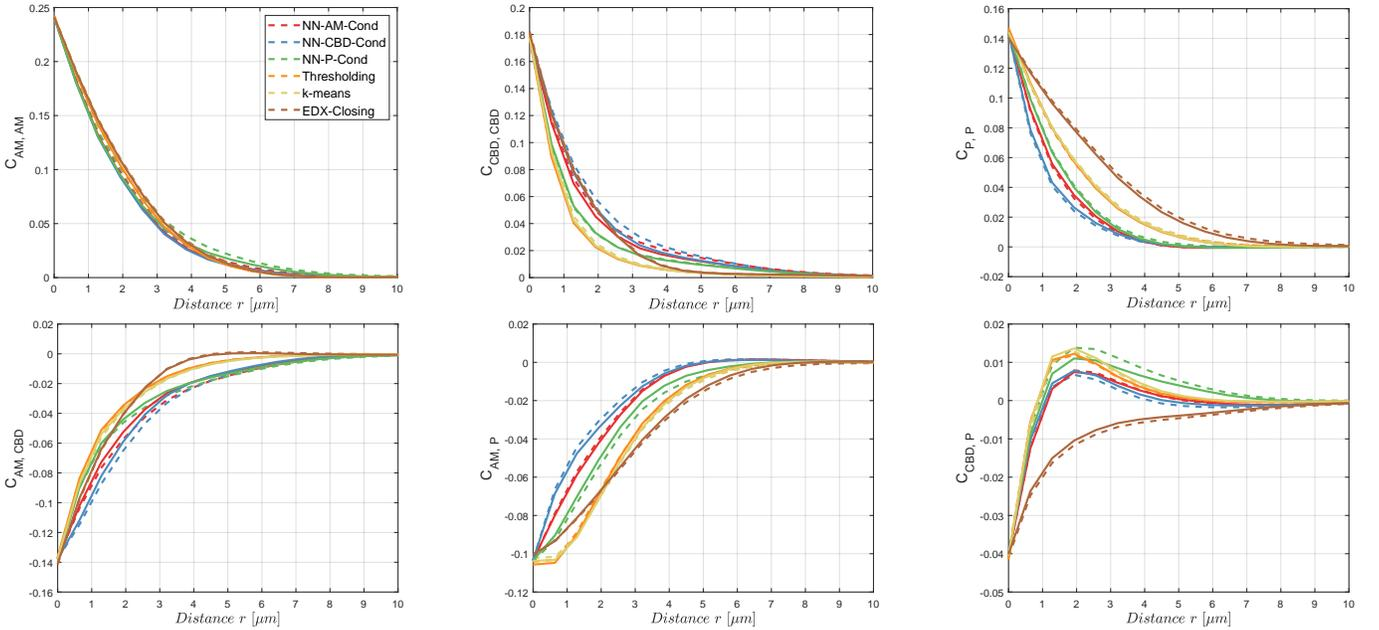
Figure 9: Top row: Centered two-point coverage probability function of active material, CBD and pore space (from left to right). Bottom row: Centered two-point coverage probability functions  $C_{AM,CBD}$ ,  $C_{AM,P}$  and  $C_{CBD,P}$  (from left to right). Note that dashed curves are used for the two-layer cathode, whereas the solid curves correspond to the single-layer cathode.
