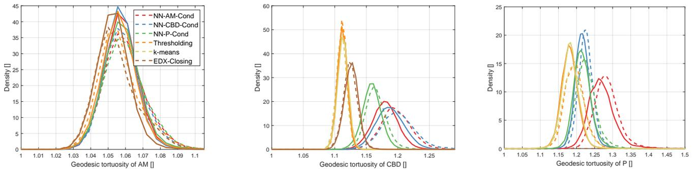
Figure 8: Geodesic tortuosity of active material (left), CBD (center) and pore space (right) for the two-layer cathode (dashed curves) and the single-layer cathode (solid curves).
