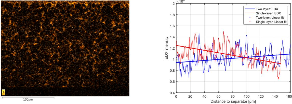
Figure 3: Left: EDX image (flourine mapping) of the single-layer cathode. Right: CBD gradient computed from EDX data (dots) and corresponding linear fit (solid line) for SL and TL.
