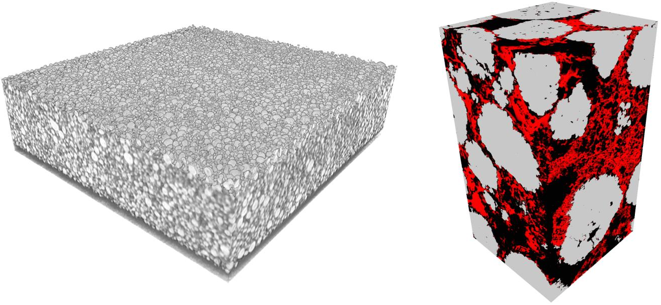
Figure 1: Left: 3D rendering of a cutout ( $640 \mu\text{m} \times 640 \mu\text{m} \times 182 \mu\text{m}$ ) of the grayscale image obtained by synchrotron tomography, where the current collector is located at the bottom. Right: 3D rendering of the trinarized FIB-SEM data ( $15 \mu\text{m} \times 14 \mu\text{m} \times 27 \mu\text{m}$ ), where active material, CBD and pores are shown in gray, red and black, respectively.
