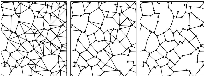
**Fig. 5** Examples of  $\beta$ -skeletons for  $\beta = 1$  (left),  $\beta = 1.5$  (center), and  $\beta = 2$  (right)
