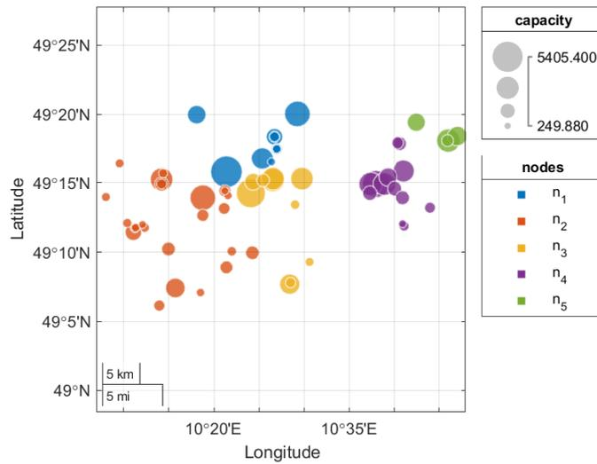
Figure 3: Locations of PV units considered in this case study, where the size of the circles corresponds to the nominal power (in kW) and the color indicates the associated network node.
