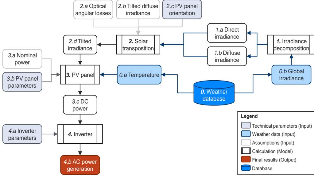
Figure 2: Outline of the different inputs, model components, parameters and the output of the physical model for photovoltaic power generation.
