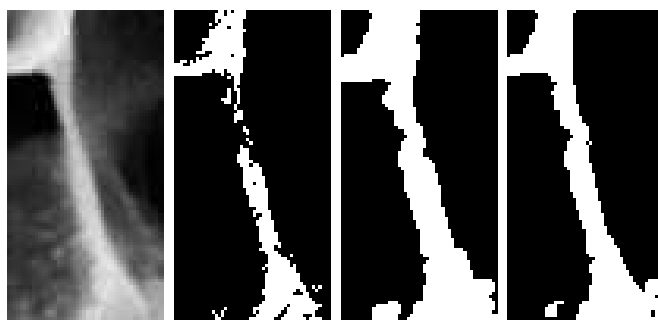
Figure 6: i) original image of cell wall, ii) result of backpropagation before postprocessing, iii) result after postprocessing (dilation), iv) for comparison: result after improvement by iterative local thresholding, which is presented in Section 5
