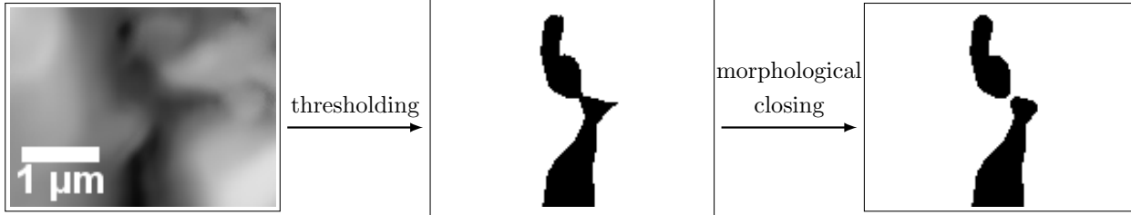
Figure 2: The procedure for binarizing a denoised image I_{\text{denoised}} (left). After thresholding the initial binarization B_{\text{initial}} (middle) is smoothed by morphological closing in order to obtain the final binarization B_{\text{pore}} of the BSE image into solid phase and pore space (right).
